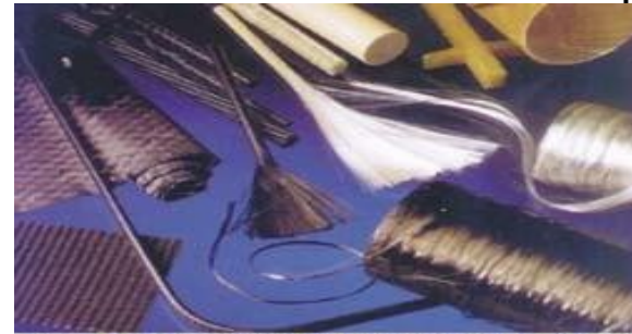
Figure 1. Common Glass and Carbon Fibers and FRPs used in Structural Engineering
