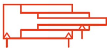
Fig. 2.34 A graphic symbol of a double-acting telescopic cylinder
