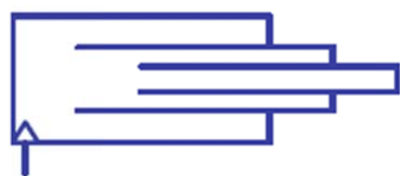
Fig. 2.33 A graphic symbol of a single-acting telescopic cylinder
