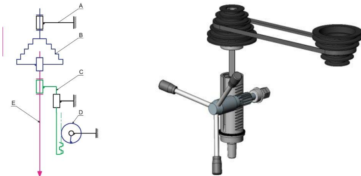
Figure III.37. Kinematic diagrams of a drill feed mechanism
