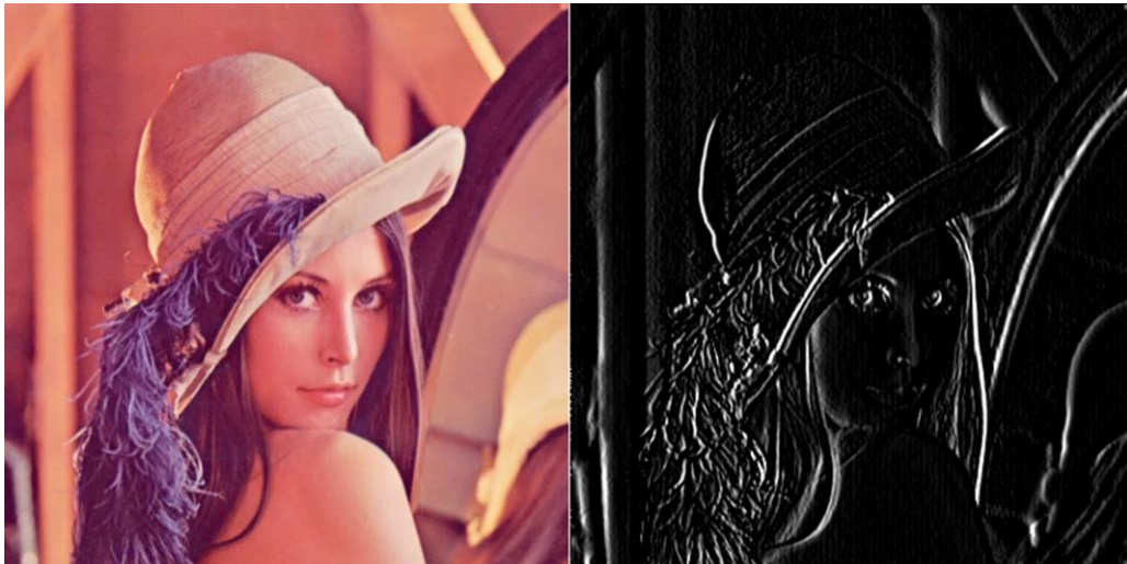
An image convolved with a vertical Sobel filter
