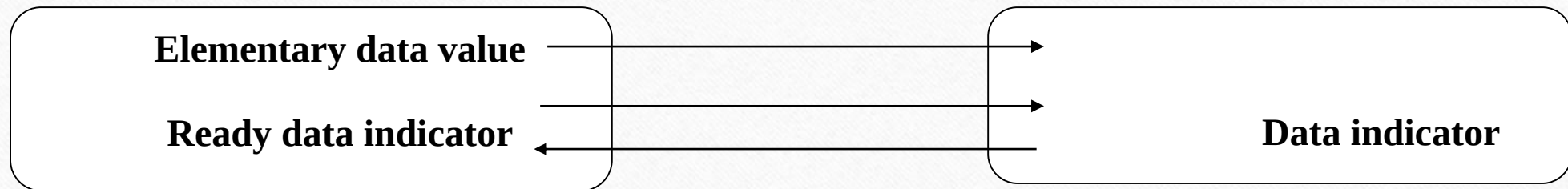
Figure 2.7 : Data Exchange Between Two Physical Components
