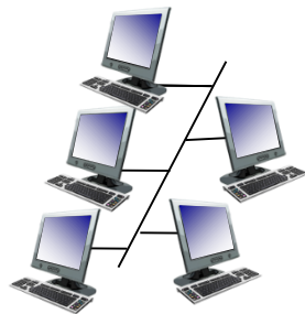
shared wire (e.g., cabled Ethernet)
